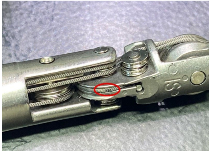
Figure G: Frayed Pitch Cable
