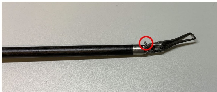
Figure F: Broken Pitch Cable
