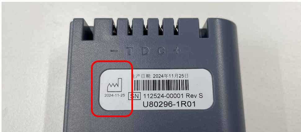
Figure 2. Example label of an affected battery. Contains Part Number “U80296-1R01”, Revision “Rev S”, manufacturing date “2024-11-25” located under the date of manufacture symbol.
