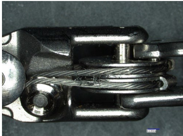
Figure D: 20x magnification of a frayed grip cable on a da Vinci Xi instrument
