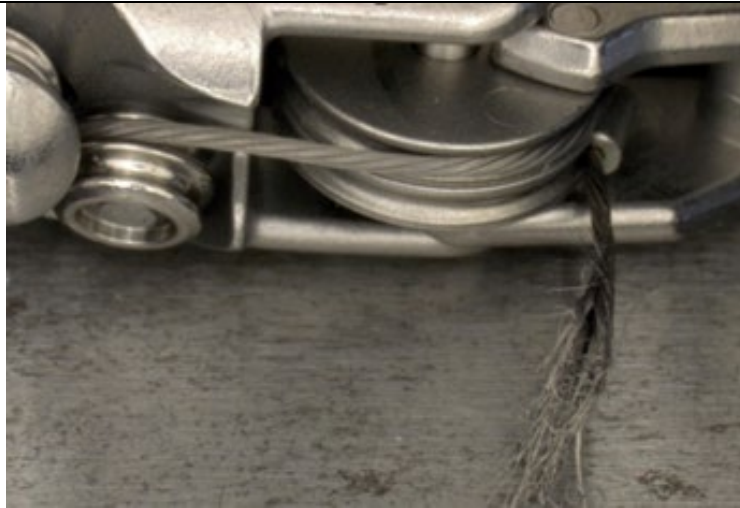
Figure C: 20x magnification of a broken grip cable on a da Vinci Xi instrument.
