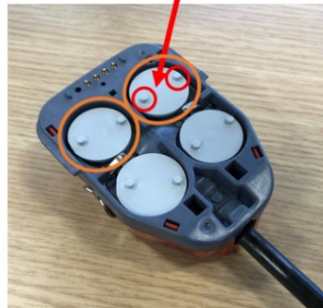
Figure 2 da Vinci S/Si Clip Applier. Sterile Adapter disc with latching holes highlighted (Left). Instrument input discs with peg features and yaw/grip discs highlighted (Right).
