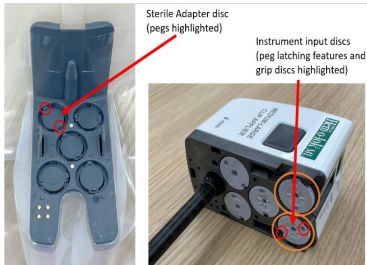
Figure 1 da Vinci X/Xi Clip Applier. Sterile Adapter disc with pegs highlighted (Left). Instrument input discs with peg latching features and grip discs highlighted (Right).
