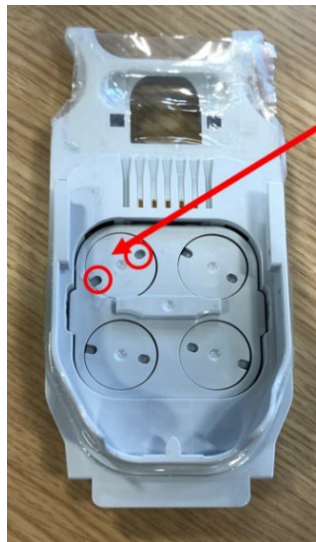
Figure 2 da Vinci S/Si Clip Applier. Sterile Adapter disc with latching holes highlighted (Left). Instrument input discs with peg features and yaw/grip discs highlighted (Right).
