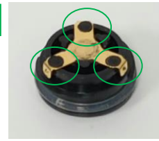
Undamaged battery cap - Continue to use Has three raised, round, black, plastic dots holding metal contact in place
