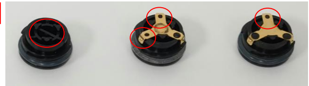
Damaged battery caps - Do not use Metal contact is missing, or fewer than 3 raised dots can be seen
